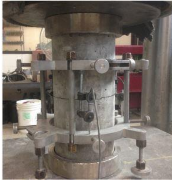
Figure 2.8: E-value Testing Arrangement for Cylinders
