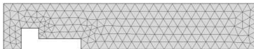
Figure: 1 Schematic drawing illustrating the two-dimensional rectangular channels along the lower wall with fixed two-step barriers at various locations.
